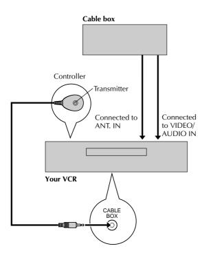
This procedure is required if you receive your TV channels through a cable box (descrambler). The Cable Box Controller allows the VCR to automatically switch the cable box channel during timer-recording. The Cable Box Controller is effective for recording shows that have been programmed using VCR Plus+ (F) pg. 40) or On-Screen Timer Programming (F) pg. 42).
